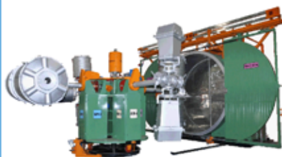
4-Arm: 4-Arm range of Bi-Axial Rotational Moulding Machines.
