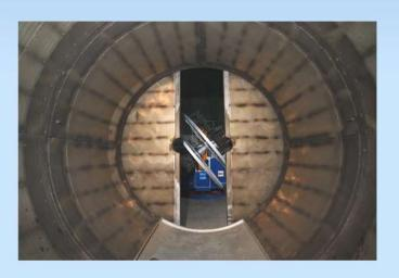
OVEN: Vinodrai pioneered in India to manufacture machines with cylindrical oven, which provides an aerodynamic geometry for highly turbulent airflow around mould avoiding hot spots. High speed twin re-circulating blowers insure upward hot-air flow resulting in considerable improve-
