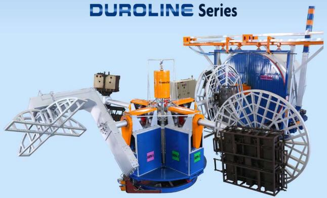
Acknowledging the requirement of our customers to produce deep cavity double wall technical parts, Vinodrai Engineers has introduced DUROLINE series of Four Arm Bi-Axial Rotational Moulding Machines.
